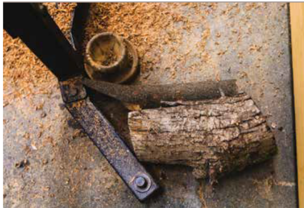
Turning creates two kinds of dust: visible dust (heavy chips that fall to the floor) and respirable dust (particles smaller than 10 microns).
