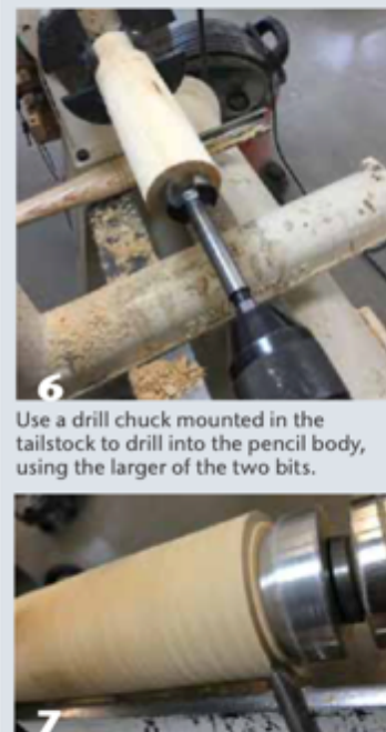
Place a cone center within the drilled hole for support and true the end.
