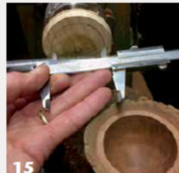
The required diameter for the lid is transferred from the bowl's rim shoulder to the lid material using a caliper.
