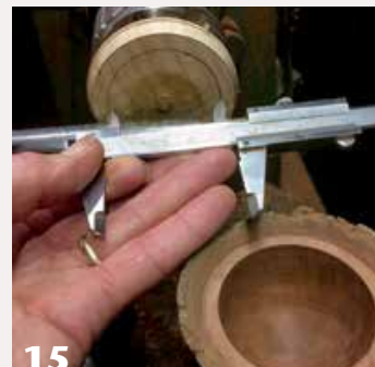
The required diameter for the lid is transferred from the bowl's rim shoulder to the lid material using a caliper.
