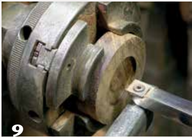
(9) A scrap of wood is held in the chuck and a shallow recess with straight walls formed. Then the author uses hot-melt glue to temporarily affix the bowl's base in the recess. Tailstock pressure is applied during gluing and the initial phases of hollowing.
