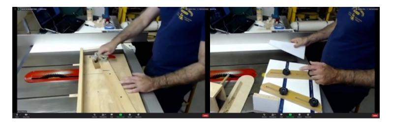
Now it's time to make the segments. Draw a line on the wood so that when you assemble it, you know top from bottom. Place the strip of wood that you are going to use on the sled (which has been set to the correct angle). Cut the pieces, alternating on the front or rear fences (for wedgie sled) or flipping the strip over for the other sled shown.
