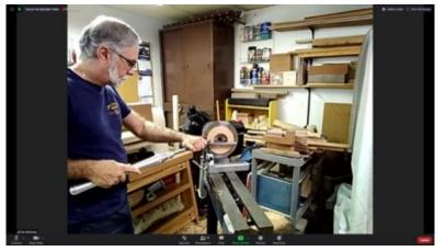
Or, attach a ring to a flat plate and put that into the chuck. Use a gouge to flatten the side.
