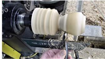
Allow greenwood surface to dry a few minutes. Remove from lathe by partially parting it. Use a saw to remove remaining stub.
