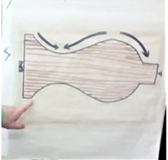
Stages to turn hollow form (2). Always turn from large diameter to small (aka downhill)
