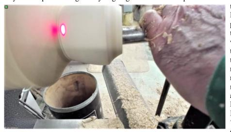
the gap between the laser and the cutter perpend to wall. As the dot falls off the wall of the piece, the proper wall thickness (gap) remains. He repeats slowly moving the cutter arm (with a fast lathe). Repeat. Listen for a light 'hiss' – it's consistent when the
