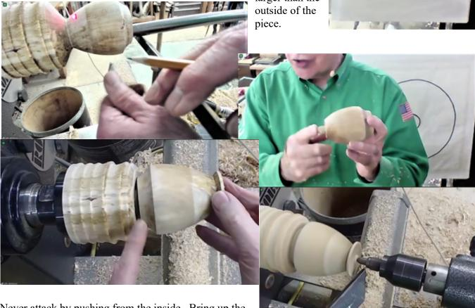
Never attack by pushing from the inside. Bring up the tailstock, making it a snug fit. Take small, light cuts to remove the remaining material from the base of the piece. Kye uses a spindle gouge to create a decorative bead on the base.
