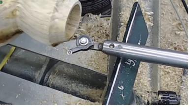
His system leans on the tool rest – always ABOVE center to produce shavings not dust. He slides the rig back and forth using his fingertips so that the hollowing jig removes the material (at '4c) in three stages"
