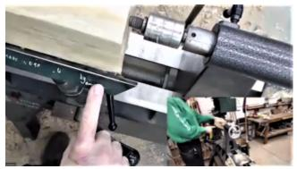
making small adjustments to find the balance point, he locks the spindle and tightens the tailstock very securely. He then adjusts his tool rest.
