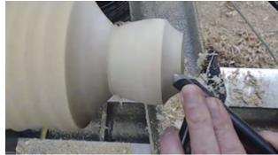
Next step is to drill a depth hole (3). Start by creating a centering cone to keep drill bit from wandering. Lyle uses an O-ring on the bit to set the depth.
