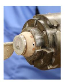
Dennis imbeds a 1" signature medallion into the base. Turn it down and remove it from the mold. Slowly drill a hole into the base of the pewter about ½" deep. Too fast and the pewter will fracture.
