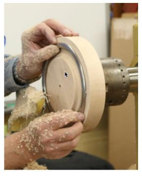
Test fit by pressing the bowl against the ring with the tail stock for two minutes.
