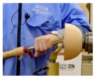
Make a friction chuck, attach some leather or a rubber carpet mat (from Home Depot) to the front, install it in the chuck.
