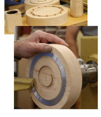
\*Unfortunately, the two tails of the liquid pewter met at a cold joint, resulting in a break.
