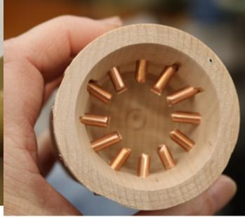
Insert the rods. Make sure no wood is loose inside the mold.
