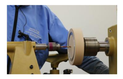
Insert a bamboo skewer into the hole to catch the ring when it becomes free. Use a parting tool to remove wood from around the ring. Hold the bowl against the ring to check size. Dennis wants it to be about 1mm larger than the bowl. Chamfer the outer edge. Now, work on the inner edge.
