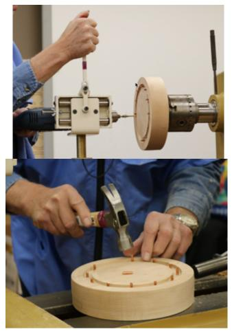
Do the same for a "foot" mold. Insert a short maple blank into the chuck. Use the tailstock for support. Use a bowl gouge to smooth the blank. Then hollow out the center, starting with a forstener bit to set the depth. Dennis suggests a 1 to 1¼" foot. Give the hollow a slight taper – wider at the top to enable the pewter to easily be removed. If using copper rods, the mold is a one-time use only.
