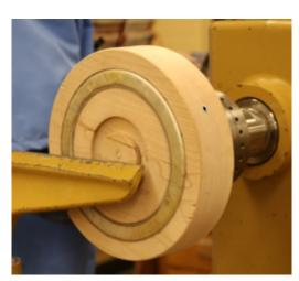
Pewter turns with the same tools as wood. However, it does not work well with a bevel cut.
