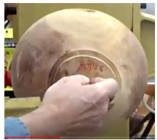
Remove the bowl, remove the little nib and reinstall the bowl. Clean up the tenon, by using a ¼" bowl gouge, to even out the tenon. Use the square scraper (raise the tool rest) with a slight inward angle (as before).
