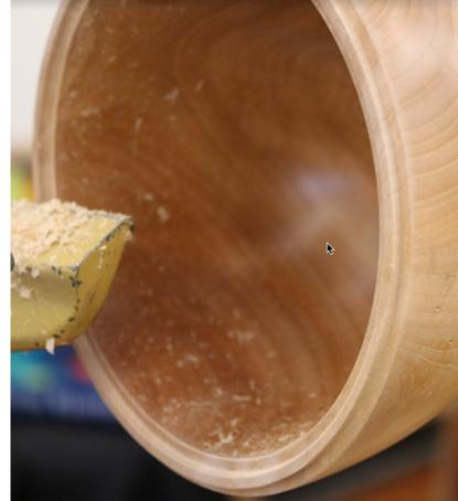
Create a mold for the pewter ring: Beginning with a disk of hard maple, mount it on the chuck.
