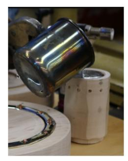
Dennis also torched the molds that had copper rods, so the pewter bonds better (also suggested, slightly sand the rods.). The pewter rose to 700 degrees before Dennis skimmed off the slag. Then poured the hot liquid into all the molds. We watched as the pewter rang around the ring to meet\* at the opposite side.
