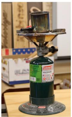
Now, turn your attention to melting the pewter: Dennis allowed the pewter to reach 700 degrees (350 to 280 degrees to melt the pewter) in a stainless steel cup. To remove the top slag, use a stainless steel spoon.
