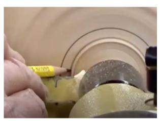
an inward sloping surface. According to Dennis, this makes it possible for the chuck to contact the bowl safely away from the inside of the tenon (at the base).
