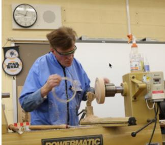
Next use a parting tool from the side to release the ring.
