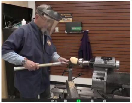
Reverse the piece onto a padded wooden fixture, bring up the tailstock and reduce and shape the tenon into a foot. Blend the bottom of the bowl into the foot. Undercut it slightly with a spindle gouge with a softened heel.
