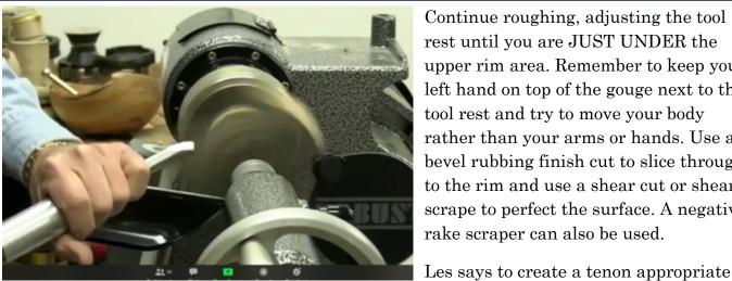
Continue roughing, adjusting the tool rest until you are JUST UNDER the upper rim area. Remember to keep your left hand on top of the gouge next to the tool rest and try to move your body rather than your arms or hands. Use a bevel rubbing finish cut to slice through to the rim and use a shear cut or shear scrape to perfect the surface. A negative rake scraper can also be used.
