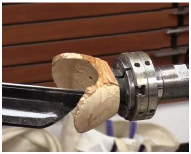
Try to make the foot 35-40% of the diameter and do not include the pith. Next, using a cedar log, start nibbling away at the bottom of the bowl.
