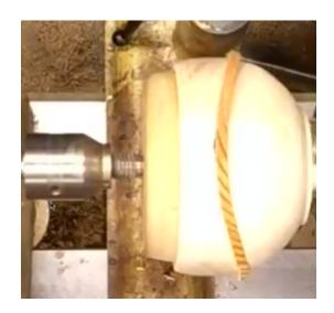
Drill a series of pilot holes to ensure you can remove exactly the same amt of material
