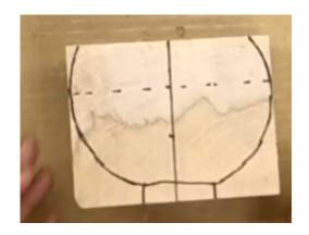
Use a compass. Set the compass to be equal to the opening of the bowl (in this case, 5"). Place the point on a temporary support block and strike an arc about ½" above and below the dotted line.
