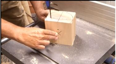
Aside: when laminating wood layers, the grain must always run in the same direction. Consequently, the veneer grain should be aligned with the block's grain. Also, ensure the endgrain also matches the same direction. Always work with North American strained grained hardwoods – avoid exotics.
