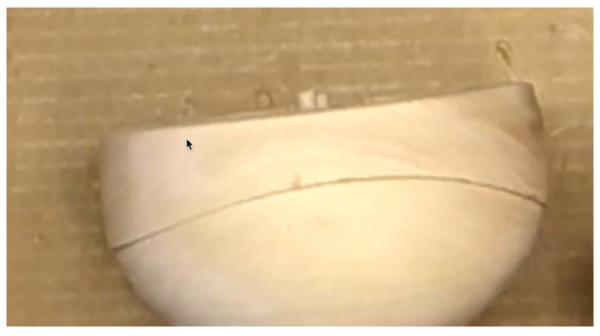
Make a spacer of the exact thickness of the gap from a soft wood. Find center. Bandsaw round. Transfer the dowel holes, drill them out. Enlarge holes. Steam (microwave) bend.
