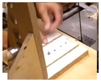
Hot glue the blocks to be perpendicular to the grain (ie align with the grain
