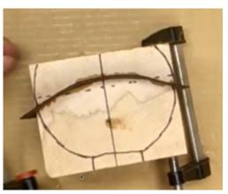
Loosen clamps and allow for airflow to really dry out the veneer. You can make a scrap block as a form so that there's no staining on your final piece.
