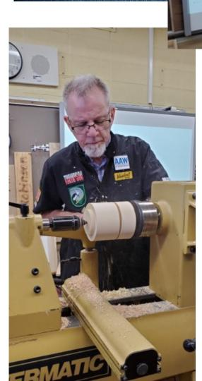
Part the two sections. Put the tenon from the bottom section into the chuck. Use the tool to clean up the tail end. Continue to remove wood, beginning at the "emphasis point" towards each end. A nice touch is the create a bead at
