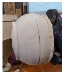
Use the skew as a scraper to remove wood from tail end inside to create a flat spot for the lid to rest. Use the spindle gouge with swept-back wings to hollow the box out. Following this, use the skew as a scraper (ie a negative rake scraper) to refine the inside.
