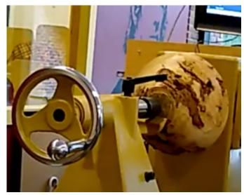
To make turning a bit easier, Mitch slid the headstock (and burl) to the end of the lathe.
