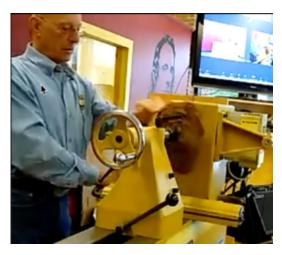
He seals the bowl (sanding sealer - shellac) before soaking it with CA to keep the CA from staining the wood.
