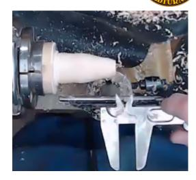
He uses a detail gouge to fine turn the end. Instead of measuring, he uses old wrenches to quickly determine sizes, referring often to his "storyboard".
