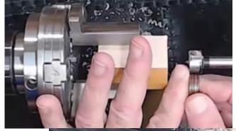
Attach blank to holder. Use a roughing gouge to round out. Match size to tenon. It helps to make a "storyboard"
