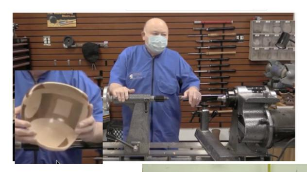
These are made from glue-ups, or from solid blocks, however, you will contend with face and end grain. For this demo, Pete used a glued-up pine block. He showed random scraps of oak glued into a block, and one made from mahogany with plywood. Out of balance glue-ups will create vibration when turned. To get the tips to be even, you must start with a cube.
