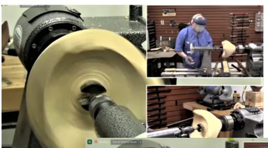
Remove the remaining center, then bore it out with a forstner bit (300 rpm) to establish the final depth of cut.
