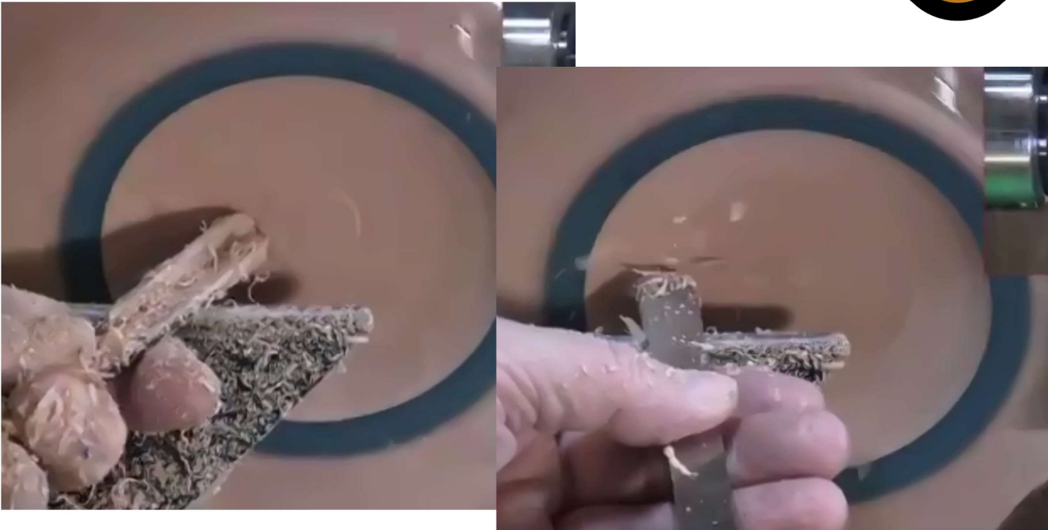
Smoothing with a negative rake scraper.
