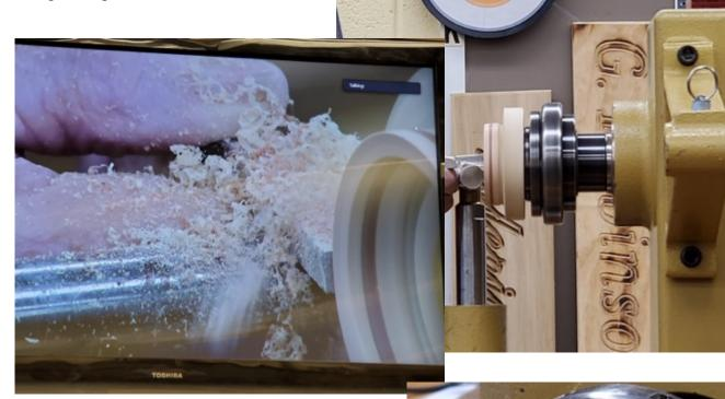
Next, he removed the block. He then reversed chucked the ring, making sure the chuck was fully seated.
