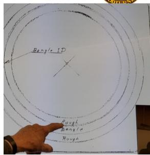
Next Bob showed how to create two bangles from the one setup: He glues another block onto ring. Then uses a parting tool to separate the ring(s) sandwiched between the blocks into two sets, each with a glue block.
