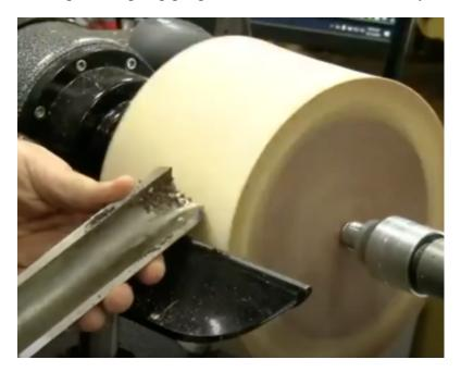
However, be careful, the part of the roughing gouge that's actually doing the cutting – ie, the part that is in contact with the wood, MUST be supported by the toolrest!
