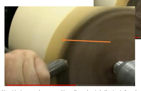
Now it's time to make a tenon. Normally, end grain hollowing is from the inside out. However, that will place a great deal of force on the outside of the bowl. Therefore, we need a large tenon. Steve uses a Megajaws chuck and wants the tenon sides to exactly match the chuck jaw angle.
