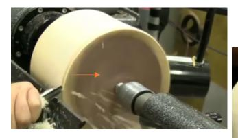
Cutting the other way results in dust, tear out and is much harder on the turner.
