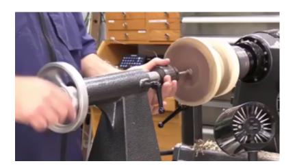
Begin hollowing from inside out with spindle gouge. This equates to working "downhill", just like using a scraper. A bowl gouge in scraping mode is an option - carefully! But NEVER a roughing gouge
