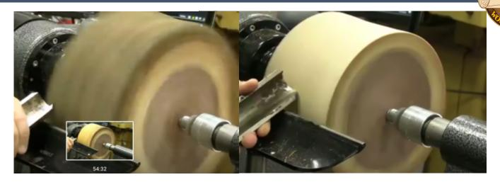
For this large piece, Steve starts by setting the tool rest above center (about ½"). The tool rest will be lowered when the diameter is reduced. Tool is locked against body at hip. Move feet and hips not arms. Lathe turning at about 700 rpm.
