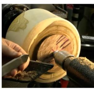
Steve does not use the chuck in expansion mode, preferring compression mode instead. In expansion mode, the hollow often defines the base of the piece. In compression mode, the foot can be removed.
