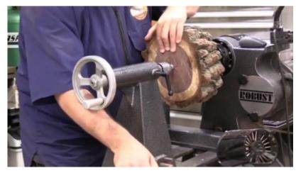
to the lathe bed, unlike if the bowl was a standard side-grain piece. Then you would never use a roughing gouge. So, here, Steve uses a spindle roughing gouge.
