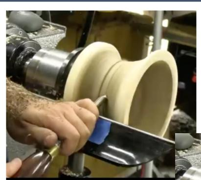
Check depth. Make mark on outside of bowl. Adjust base accordingly. Switch to spindle gouge. Adjust tool rest as needed.
