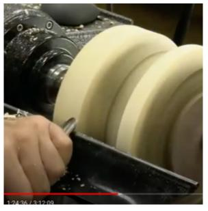
Remove some material to provide a visual shape for later hollowing.
