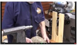
For large blanks, you can use a One Way "big bite" drive. A face plate is the most secure, but can't re-position the blank. The Elio Drive, available from the Woodturning Tool Store, is his go-to.
