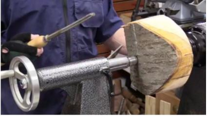
Rubbing the bevel Shear scraping Negative rake scraper
