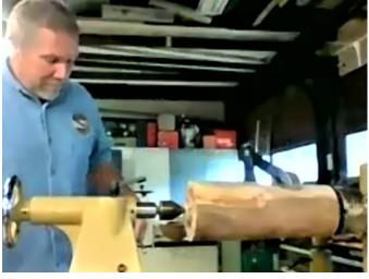
The bottom tenon gets removed and trimmed to provide access for hollowing (and later it is reattached).
