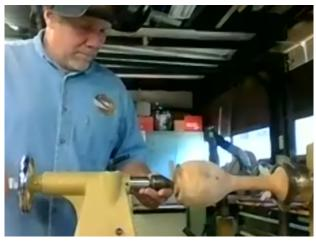
He then reversed the vase and removed the other tenon. He used another forstner bit to hollow all the way through, intersecting with the first tenon. Using "very light cuts", Henry finished the outside, refining the shape. (BTW, that's a bamboo extension Henry made.)
