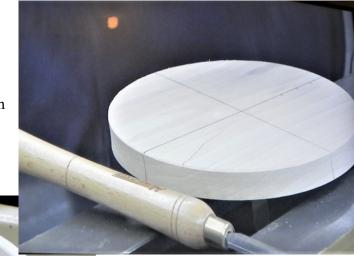
Mark concentric circles as shown. Set an angle gauge to 50 degrees and place it on the toolrest to aid in aligning the cutting tool.
