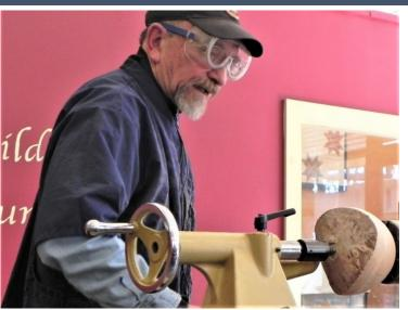
Return tool rest to back of bowl and create tenon to fit chuck or flatten to fit face plate. Tenon can be straight or dovetailed to fit jaws. Can create dovetail by raising tool rest and using skew on its side.
