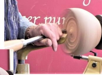
slightly hollow the base. Sand the foot. Remove from lathe, cut remaining nub with a wood chisel and sand smooth.
