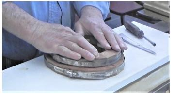
Next, assemble the segments into a ring. Place blue tape (sticky side up) on the table. Begin with one segment (the short side of the segment faces up), place it on the tape. Repeat with each segment (make sure the edges are tight to each other). Quickly put glue on each adjacent piece. When done pick up one end of the tape and move to towards the other end, turning the pieces into a ring (be sure to glue the first and last pieces).
