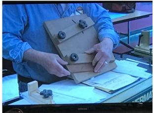
• After that, you place the wood on the sled and slide it through the blade. If you use a homemade zero clearance table saw inset which has a deflection guide on it, the pieces fall away from the blade after cutting. Move the piece to the adjacent fence and repeat (see photos). A light sanding to remove the fuzz is all that remains.
