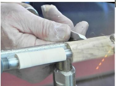
Adjust the tool rest. Barry prefers to use a skew, held so that the lower 1/3 is held at an angle to the wood, but some turners like the roughing gouge or spindle gouge, to round the blanks. Take care to not cut into the spacers.
