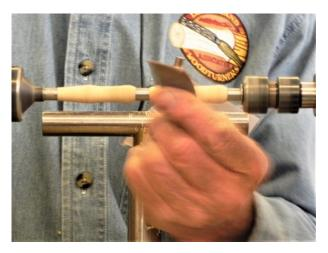
Remove the metal bushing and replace with nylon one supplied in the kit. This will prevent the CA finish from sticking.
