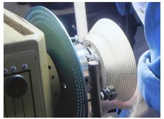
In use, the jig (pencil) is held against the bowl, which has been indexed. Draw a line from bottom to top, rotate the bowl to the next indexed mark and draw another line. Repeat until the bowl has returned to the original line. You've created rectangles on each bead. Choose the number of rectangles to make a pleasing arrangement (of course you are working off your original plan).
