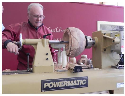
Don talked about the advantages of coring bowls - less waste of wood, fewer shavings to dispose of and production of nested bowls. He demonstrated the use of the Woodcut and Oneway systems which have their pivot points located out of the bowl versus the McNaughton system which has a virtual pivot point. He showed how the McNaughton can yield deeper bowls than the other two but may be more difficult to use.
