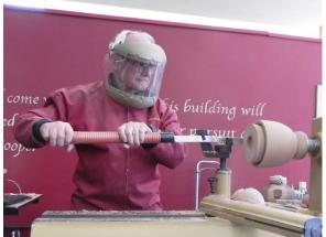
the groove, especially to prevent catches when coring a burl or natural edge bowl. When coring the outside bowl first, Don leaves a mortise in the center of the blank to help in mounting the inside bowl.
