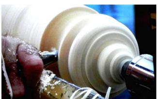
emphasized riding the bevel for safe clean work. Start with the handle down and raise the tool until it begins to cut. He switched to a spindle gouge and showed the same technique keeping the tool at the center of the workpiece. He grinds the heel of the tool to create a secondary bevel which gives him greater clearance in tight spots.
