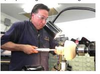
He started hollowing using his 55 degree bowl gouge, keeping the tip on or slightly lower than center, starting from the
