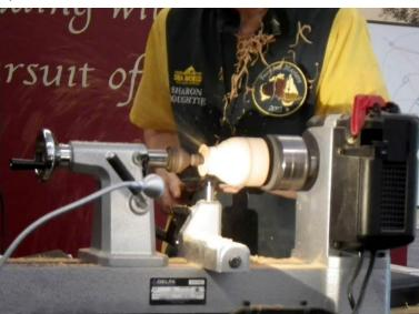
Placing the top in the chuck, she trued the blank and then used a detail gouge with a 40 degree long bevel to partially shape the outside into a teardrop shape and to hollow the inside. The inside was then sanded and a 1/4" motise was created and trued so it was parallel to the lathe bed. She then placed the
