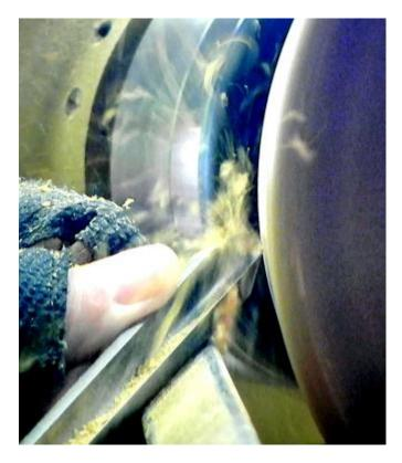
The bowl gouge can be used as a scraper to create a tenon or to flatten the bottom of a bowl.
