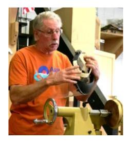
After shaping the outside of the bowl, John turned it around and hollowed it with a gouge. He suggested drilling out the core to make it easier. John hollowed from the larger diameter to the center and first cut a set of starting ridges to keep the gouge from skating.
