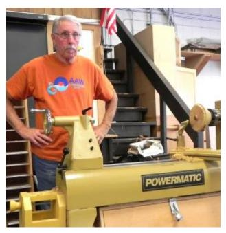
Tool rests should be filed flat or use Robust toll rests with hardened steel bars. Set the rest and hand turn the blank to be sure it doesn't touch. The rest should be set so that the gouge's flute will be on center.
