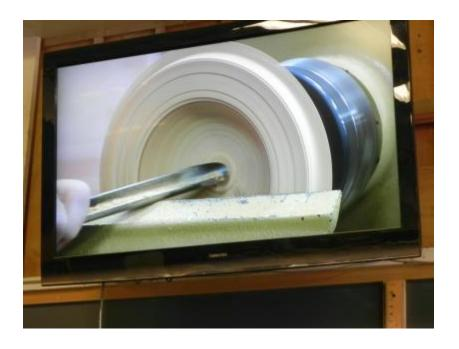
He uses a 75-80 degree gouge to do the bottom of the bowl. When using a scraper, round off the bottom edge of the tool shank so it slides easily on the rest. Use the tool pointed down, (raise the tool rest), and scrape with the burr on the end of the bevel.
