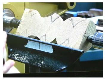
When attempting a new design, Mark suggests laying out 2 blanks and keep precise notes of the turning procedures and the dimensions of the final cuts so they can be duplicated.
