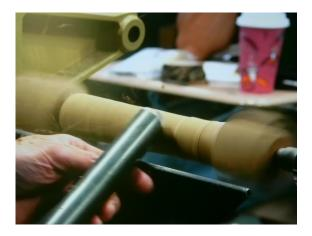
He uses a Thomson 11/4" roughing gouge ground to 30 degrees. He uses a 5/8 bowl gouge with a deep flute for cleaner cuts when making coves in his multi-axis pieces.
