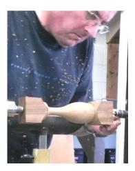
Mark uses cup centers (Oneway center with a spring is recommended) on the drive and tail ends both for safety and for ease in changing axes. He also recommends Robust tools rests.
