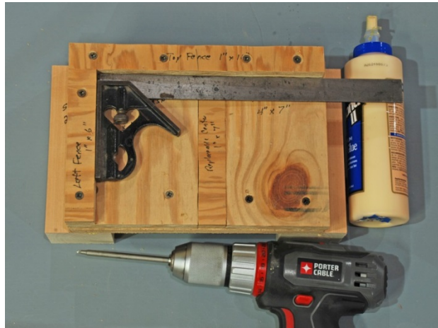
Figure #6: After attaching the fences to the Drilling Jig.
