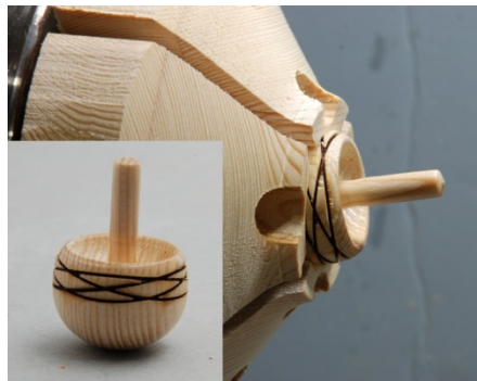
Figure #27: Adding decorative burned lines to the top with tippy top jaws.
