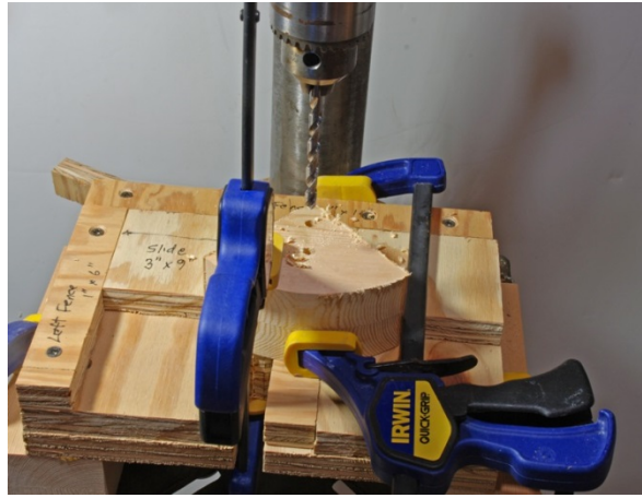
Figure #18: Drilling body holes from the bottom of the Blank with the smaller drill.
