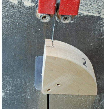
Figure #28: Cutting a rebate for the handle in one of the jaws.
