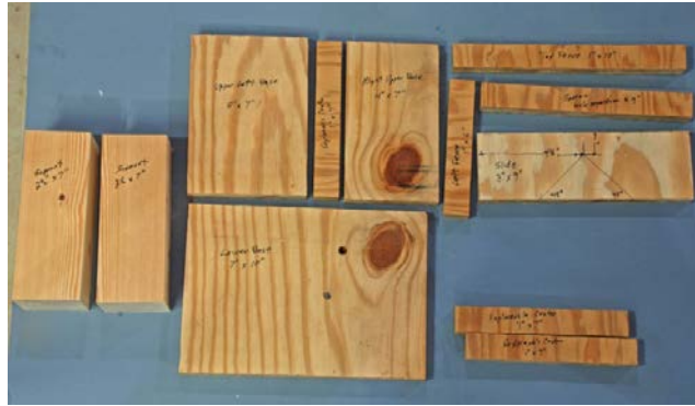
Figure #2: The parts for the drilling jig after cutting to size.
