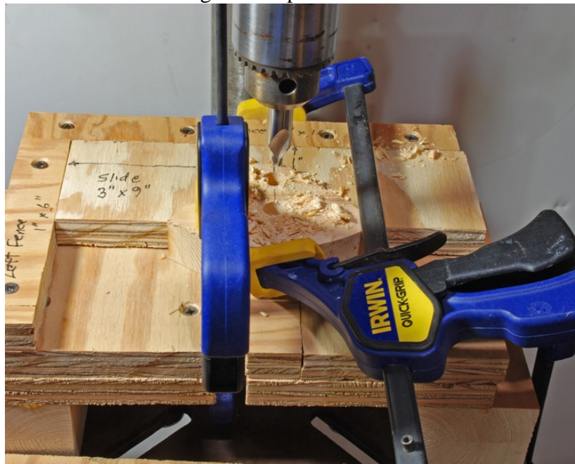
Figure #16: Drilling the outer hole in the Jaw Blank.
