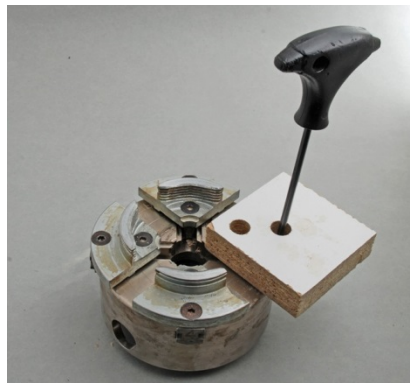
Figure #14: Testing the hole separation by mounting the test scrap on the chuck.
