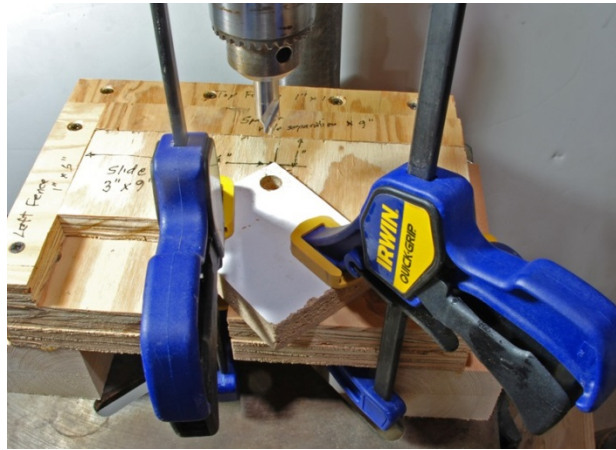
Figure #11: Testing the drill press depth stop by drilling a test scrap.
