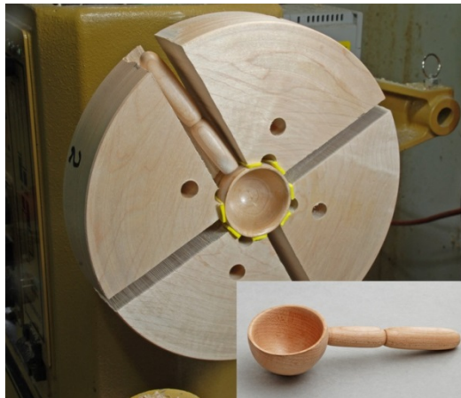
Figure #31: The set up for hollowing and completed scoop.
