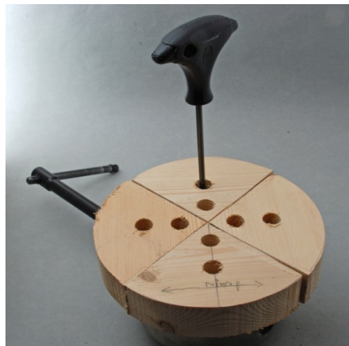
Figure #21: Tightening the jaws after closing them.
