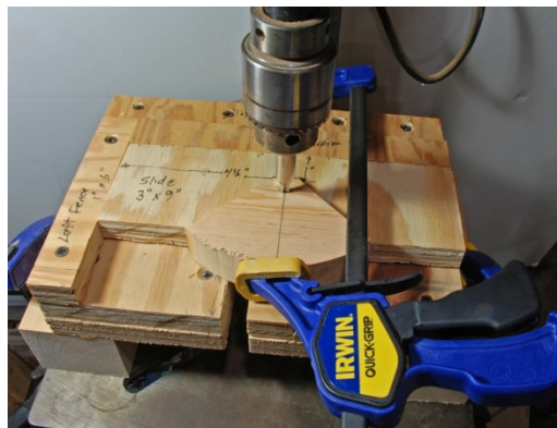
Figure #10: Locating the Drilling Jig on the drill press.
