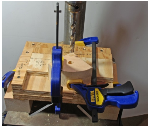
Figure #19: Counterboring from the top of the Blank with the larger drill bit.
