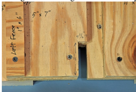
Figure #7: After cutting out a clearance notch for clamps.
