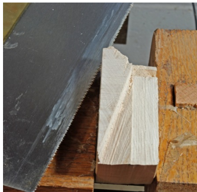
Figure #29: After cutting a ramp with a hand saw so that the handle can be angled.
