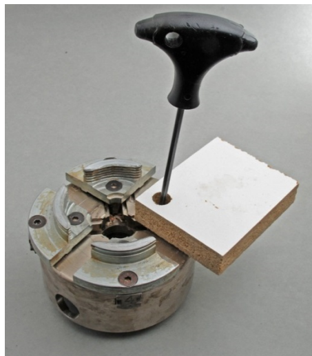
Figure #12: Testing the countersink depth on the chuck.
