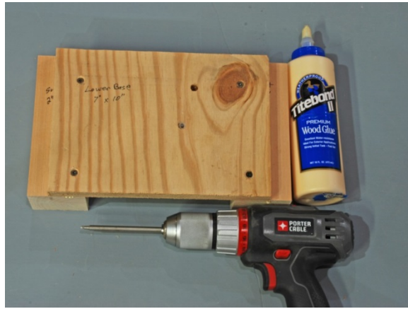
Figure #4: After attaching the Lower Base to the Base Supports.
