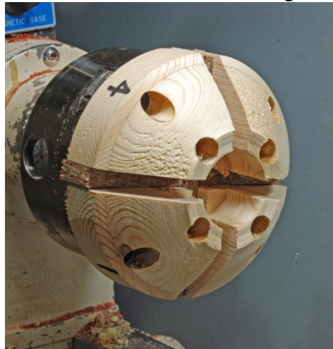
Figure #26: After shaping tippy top jaws.
