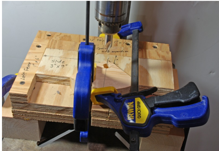
Figure #15: Drilling the inner hole in the Jaw Blank.
