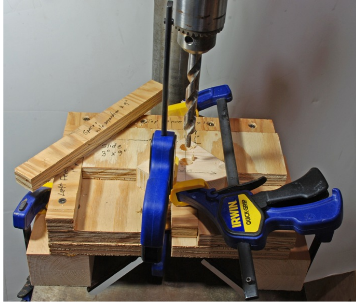
Figure #17: Drilling and countersinking in one step using a Subland drill bit.
