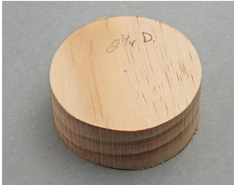
Fig02: The cone blank, a 2-3/4" disc of wood about 1-1/8" thick.
