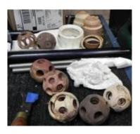
Don started with 2 ¾ square by 6" blank which he rough turned to a 2 ½' "cylinder. He suggests using Fred Holder's book and using a digital caliper for all measurements. A cup chuck is used to turn off the nubs on the balls and the end grain is marked. He turns several balls at a time and soaks them in Cedar Shield. Using a compass set at 1.3190" he scribes circles on the balls marking first the N end and S end and then, taking an arbitrary point, scribes circles that intersect to lay out the 12
