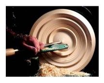
He progressed to the center removing wood until a four to five inch circle remained. Les explained that this small center circle could be utilized to carve a design ,i.e. animal, tree, flower in this space to enhance the overall effect and design of the turning.
