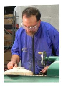
Using a one-half inch gouge, a vee notch was formed on the outer edge.
