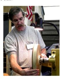
It is a good idea to mark one of the radial lines as top and mark each ¼" doughnut while it is on the lathe the first time. The inside hole of each doughnut is lined with plastic tubing cut along its length.
