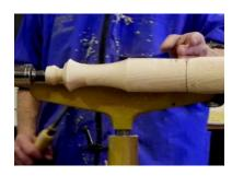
Using a sharp parting tool, the male dimension was sized to fit into the female top section.
