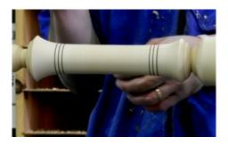
To finish the box, Joshua uses an abrasive wax compound. For added detail, he will sometimes burn decorative lines to hide the seam line of the two sections.
