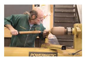
Rich began his demonstration by mounting a six inch by ten inch blank of walnut between centers. He formed a tenon with a bowl gouge and then mounted the blank in a chuck.
