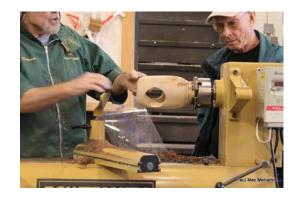
Rich will finish cut the top section of the vessel before proceeding down to the bottom. He explained that it is very difficult to return to the top portion after it has been turned to a thin dimension.
