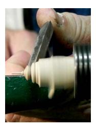
Alan began his demonstration by "warming up" and turning tiny spinning tops tops with a 1 ¼", 3/8" thick skew chisel. These completed tops were 3/8" high and approximately ¼" wide. Alan showed that such a large and heavy tool, when properly used, could yield such a small well-turned result.
