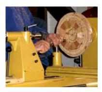
With the lathe now running, Charlie flattens the face of the ring using including a gouge and round nose scraper.
