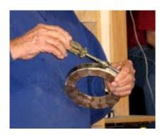
Glue and clamp two segments together making one two-piece segment.
