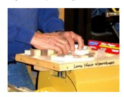
Next, glue each two segmented piece to another make a four segmented section of the ring. Continue to glue sections of a ring until the desired number is reached. For this demonstration, Charlie used 24 segmented for each ring.
