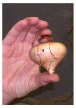
John Kowalchuk was the third demonstrator of the day. John turned a birdhouse ornament consisting of a hollow base that was drilled in two areas. One hole held the perch and the other simulated the entrance to the birdhouse. The top was a conical shaped piece of contrasting wood for a pleasing appearance. Pear wood was used for the base and spalted maple for the roof.
