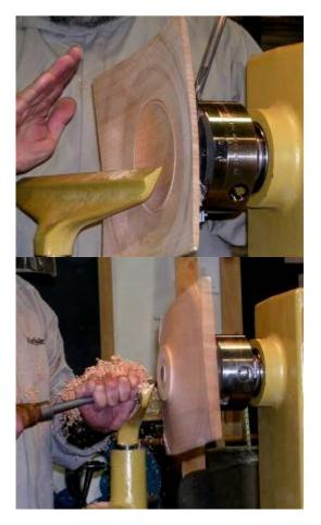
Power sand the rim out to the edge (not the corner) with the lathe running. Turn off the lathe to blend in the corners. All uses a variety of backings when power sanding, they can be hard backing or foam and the foam can be firm or soft. All finishes the bowl by texturing the rim. The texture in this case was created by drawing a series of concentric circles and radial lines. All then power carved each line segment.
