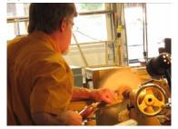
The piece was mounted between centers and trued both ways. He used a swept back "Ellsworth "type grind for this task."
