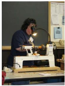
Melissa began by turning the finial. After truing the blank, she used a 3/8 "spindle gouge to shape the finial. For optimum stability, Melissa urged turners to keep as much material near the blank as possible.
