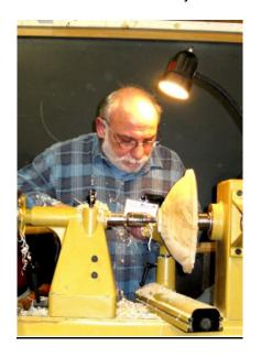
Joel stressed to position the scraping tool at or below the center line of the bowl. Using the shear scraper above the center line will result in a serious catch which could ruin the piece.
