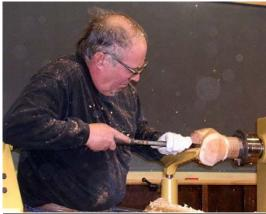
On the inside section of the bowl, Lenny used a sander with a flap wheel. If he encounters a small split in the wood, Len will use a burning tool to disguise the crack.
