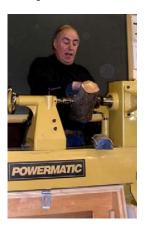
Len began turning by rounding the long end. He emphasized to look at the shape being cut-don't focus only on the cutting made by the cutting tool. Once the final outside shape was roughed, Lenny began hollowing the bowl side.
