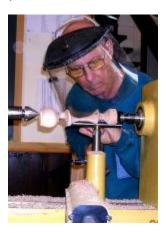
Off center or multi-axis turning may be done by working between centers with a spur drive and tailstock or using a special eccentric chuck.
