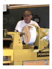
After the outside shape was completed, Jim reversed the bowl again mounting the bottom tenon in a chuck to hollow the inside of the blank.
