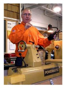
A good stance at the lathe, sharp tools and proper technique is essential to producing well turned projects safely.
