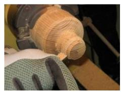
The tool is presented to the wood, again using a slow speed, in a back and forth, slightly circular motion. This insures that the threads will be cut uniformly.
